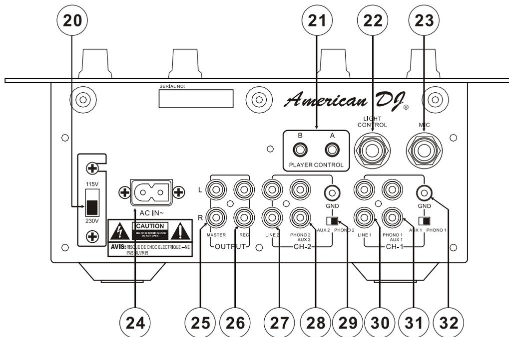
**20. AC VOLTAGE SELECTOR** - This switch is used to adjust the operating voltage. Operating voltage can be toggled between 115V/50Hz or 230V/60Hz. Always be sure the selector is set to the proper voltage for your area before attempting to operate the unit.
