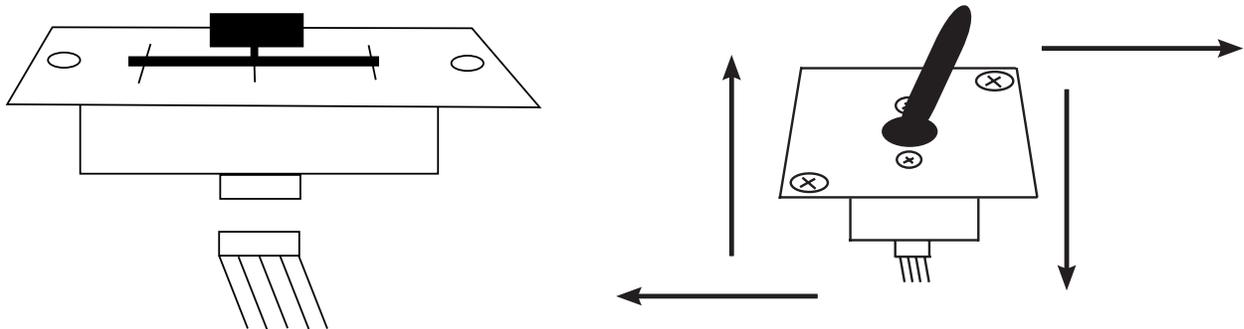
The crossfader is “Hot Swappable” which means it may be replaced at any time, even when power is applied. Only replace with American Audio Part Feather Fader Plus. Replacing with any other model fader may seriously damage your mixer.
